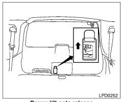
Power lift gate release Power lift gate (if so equipped)
